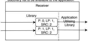
Multiple sources can be sending discovery packets simultaneously. Here 2 sources have sent the first page.
