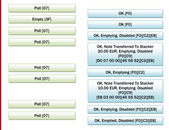
An OK (0xF0) response to the empty or SMART Empty commands indicates the empty operation was accepted and will begin. The following error codes could also be returned.
