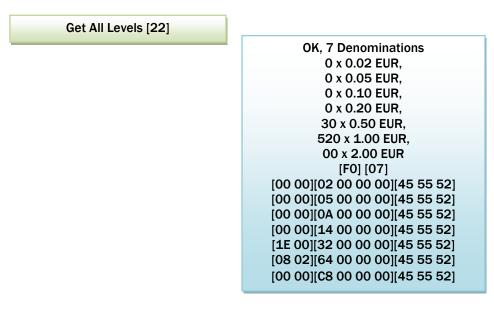
For both of the level commands detailed above, if the payout unable to process the command, Command Cannot Be Processed (0xF5) will be returned.
