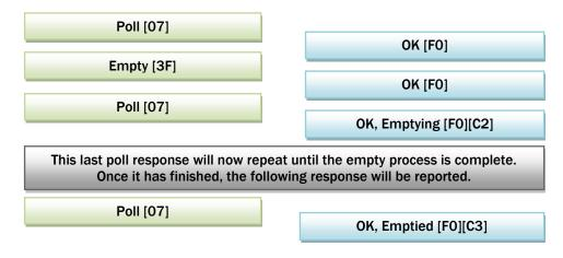
The device will respond to Empty command (0x3F) and SMART Empty command (0x52) with OK (0xF0) if there are no problems. Alternatively if the command was sent unencrypted then Parameter Out Of Range (0xF4) will be returned.
