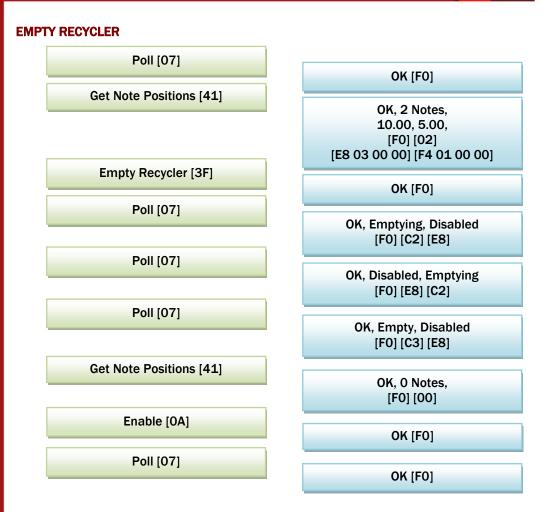
The device will respond to Empty command (0x3F) with OK (0xF0) if there are no problems. Alternatively the following responses could be received:
