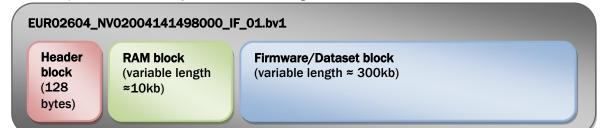
The **Header block** contains details about the file including validator type, versioning information and download configuration data used by the validator during the update.
