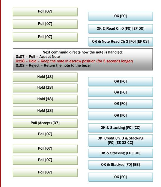
If there is not a note in the escrow position and the host sends Hold command (0x18) the device will respond with Command Cannot Be Processed (0xF5).
