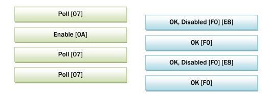
Enable will always respond ok, use Poll command (0x07) to check the SMART Hopper has enabled. The Disabled event is reported for one Poll response after the Enable command is received. This is so that the host is informed the device has been disabled.
