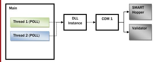
There is only one channel (port) the data can go through to the SMART Hopper and the validator. If SSPSendCommand method is used by both threads without the first call completing and a response being sent back, it will not work.
