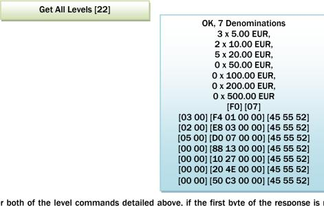
For both of the level commands detailed above, if the first byte of the response is not OK (0xF0) the possible error conditions are as follows.
