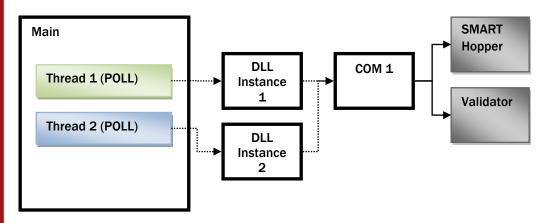
This is not possible as there is an internal flag in the DLL that requires that instance of the DLL to open the port before commands can be sent. This would mean both instances would have to open the port and this is not possible. There is not currently a way to pass/get the open port handle in the DLL instance.
