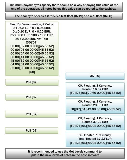
As with dispense commands, the response can potentially return a Command Unable To Be Processed (0xF5) response with an error byte detailing the cause of the error. See details in the payout section above.
