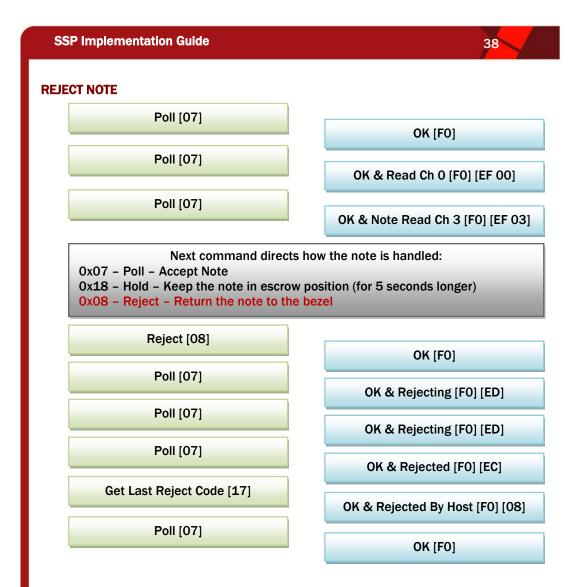
If there is not a note in the escrow position and the host sends Reject command (0x08) the device will respond with Command Cannot Be Processed (0xF5).
