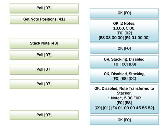
The device will respond to Stack Note command (0x43) with OK (0xF0) if there are no problems. Alternatively the following responses could be received:
