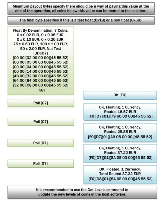
As with dispense commands, the response can potentially return a Command Unable To Be Processed (0xF5) response with an error byte detailing the cause of the error. See details in the payout section above.
