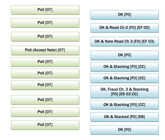
When a fraud attempt is seen as part of the note reading process it is usually because the validator has detected something is not as it should be. It is recommended that they are always logged as part of the host security log.
