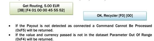
If the command was sent unencrypted then Parameter Out Of Range (0xF4) will be returned.
