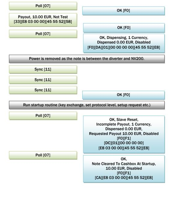
If the power is removed once the note is inside the NV200, but not yet reverse validated and being returned to the customer; the flow will be as follows.
